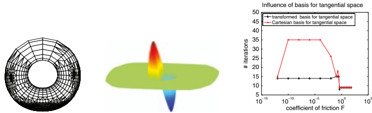
Fig. 1. Torus in contact with a rigid foundation Left: Deformed geometry. Middle: First component of the tangential stresses. Right: Block on plane: Robustness w.r.t to the coefficient of friction. Influence of coarse grid spaces \mathcal{X}_{\bar{\mathbf{u}}^L}^\ell
