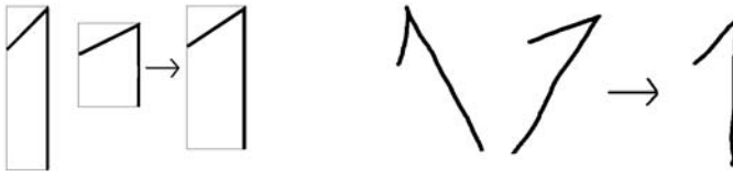
Fig. 2. The result of using scaling (on the left), and rotation removal (on the right) algorithms
