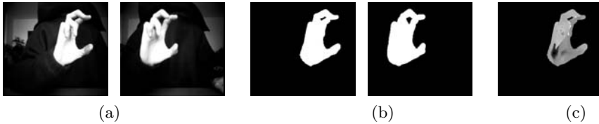
Fig. 3. Hand areas (b) detected for the pair of stereo images of Ch model posture (a) and the depth map obtained for this posture (c)
