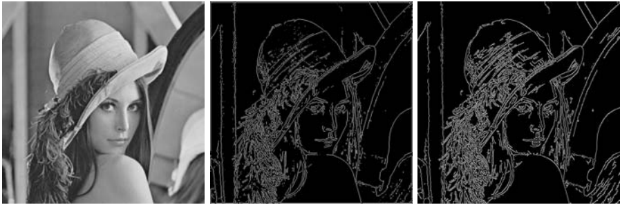
(a) Original test image (b) Morphological edge detector result (c) Canny edge detector result
