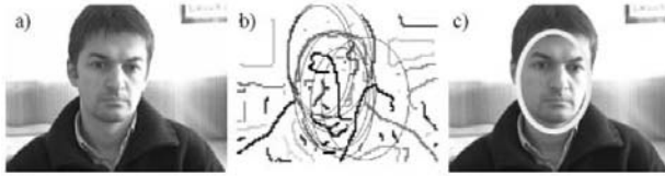
Fig. 1. The method of edge maps: (a) source image, (b) final form of the edge map with candidate ellipses, (c) localized face
