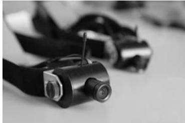
Fig. 1. The WearCam, a 60 grams head-mounted wireless camera
