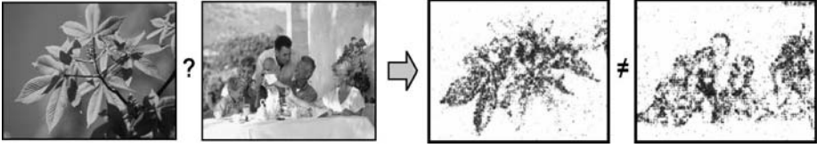
Fig. 5. Candidate verification. Low-pass of phase correlation bases the image comparison on their major edges.
