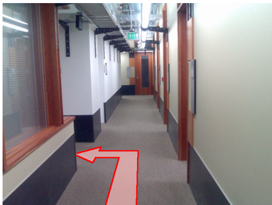
Fig. 10. This shows an arrow overlaid to match the perspective of the floor. The calculated homography was used to place the arrow.
