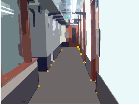
Fig. 3. The hallway image is first segmented with Mean Shift, then the edge of the floor traced and corners located. Corners marked with orange circles are candidates for matching to floorplan features.
