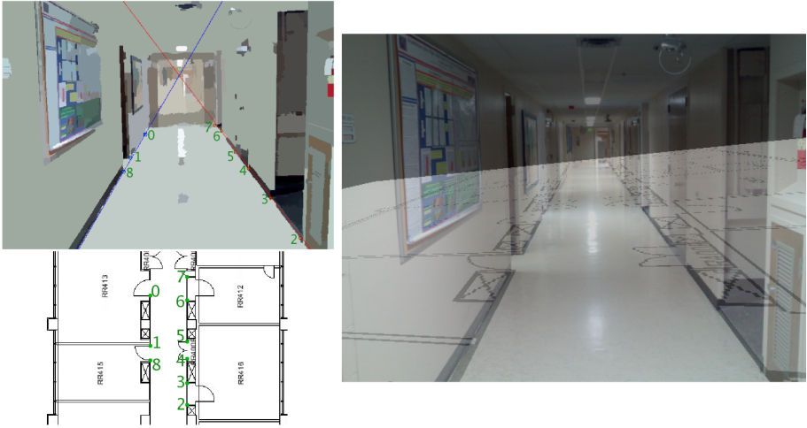
Fig. 7. Results of point correspondence algorithm. Upper left: the detected points on the image labeled by number. The detected points of this example required some manual filtering to get a good match. Lower left: the points on the floorplan that were matched to the image, labeled with corresponding numbers. Right: floorplan warped into the image space and overlaid on top of the original image. This example has 9 image points and 19 map points and completes matching in about 8 seconds.
