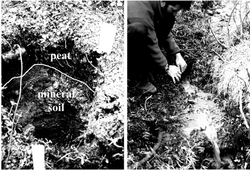
Fig. 7. Two-layer flow system, Wolf Creek basin, Yukon: (left) peat overlying mineral soil on a subarctic north-facing slope, (right) quick flow in the peat layer demonstrated by an outpour of water when the peat is lifted. (Photos: S. Carey)
