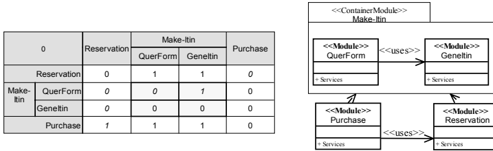
Fig. 2. The architectural modular view for a ticket purchase-reservation system, in relationship matrix and UML 2.0 representations
