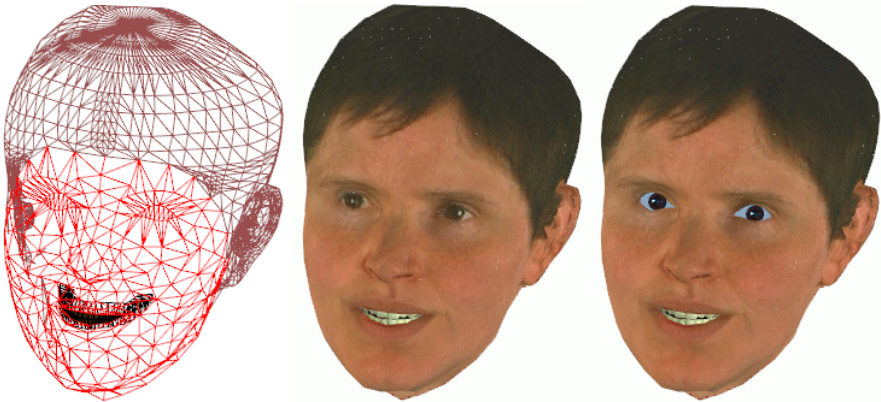
Fig. 5. Our virtual talking face is driven by 12 facial degrees-of-freedom [2]. The eyes and eyelids movements are controlled by 5 degrees-of-freedom that capture the correlations between gaze and eyelids deformations [3].
