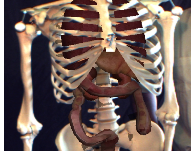
Fig. 4. For a realistic impression of augmented reality virtual objects have to be occluded by real ones
