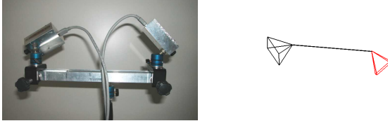
Fig. 5. Photo of real rig (a) and 3D model of the rig calibration estimate (b)
