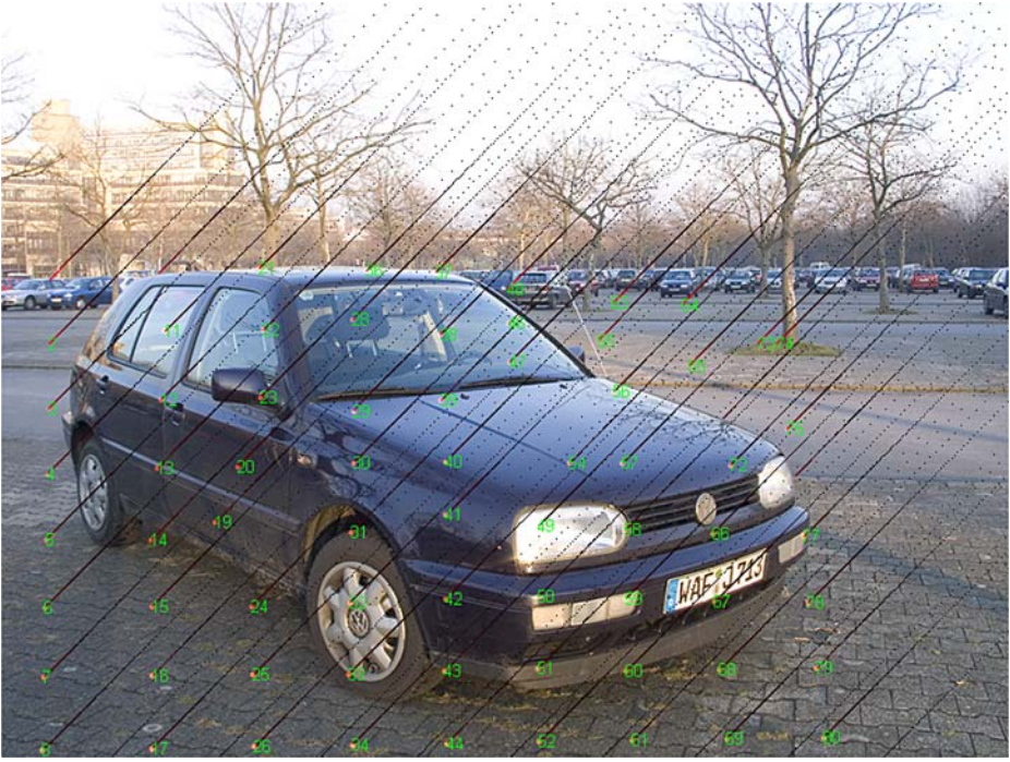
Fig. 5. Modified projection pattern with specified 5 pixel minimum distance
