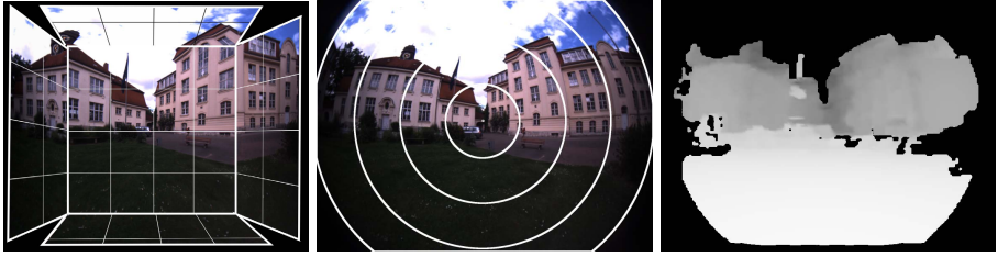
Fig. 1. Left: 3D view of cube-mapped environment (perspective views) Middle: Fish-eye image with center, 45°, 90°, 135° and 180° field of view circles, Right: Example of Reconstructed Fish-eye Depth Map
