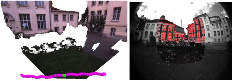
Fig. 5. Left: Perspective view on reference model and extent of camera movement used for drift measurement. The camera is going forward/backward from one end of this path to the other. It passes the green middle camera, where the pose estimation is compared to previous and following passes (see table 1). Right: augmentation of model view and real image using estimated parameters. The texture used for the augmentation is the gradient magnitude of original texture, strong gradient edges colored in red.
