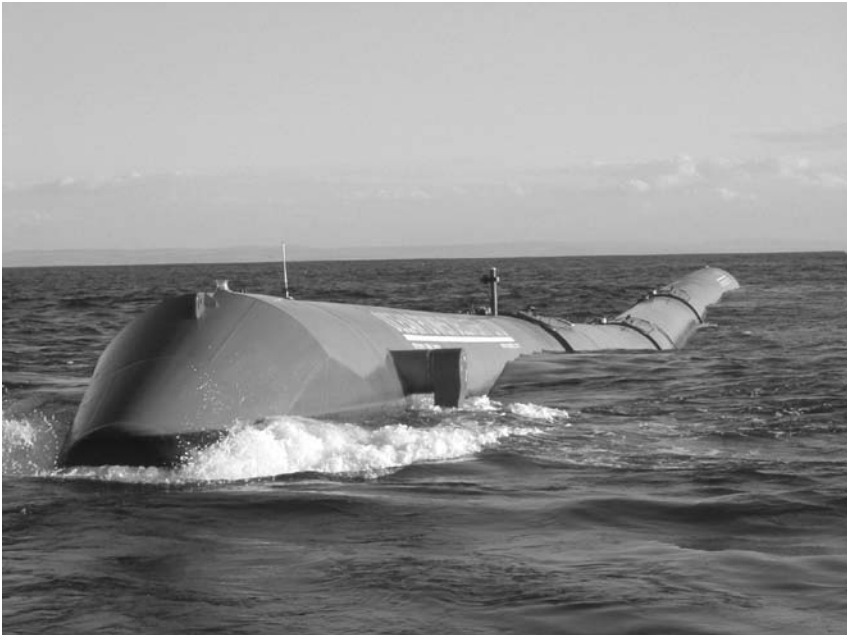
Fig. 7.17. The Pelamis WEC full-scale prototype (150 m long, 3.5 m in diameter)
