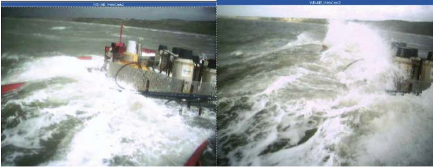
Fig. 7.75. View from web camera mounted to the device's shoulder of waves crashing into turbine area
