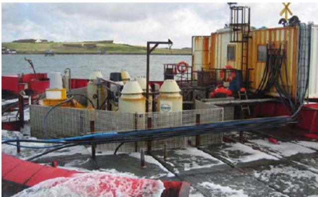
Fig. 7.81. Trash rack with 5 \times 5\text{ cm} grid openings enclosing the turbine area
