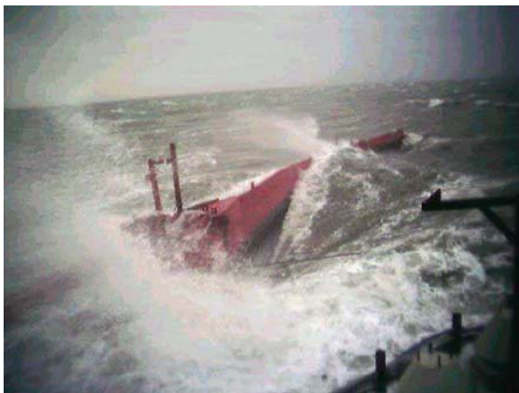
Fig. 7.74. View from web camera mounted to control container of large wave surging down reflector wing of Wave Dragon
