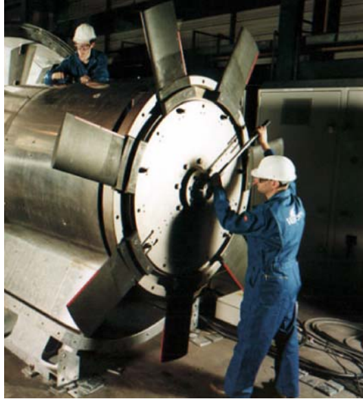
Fig. 7.2. Wells turbine used in the LIMPET plant
