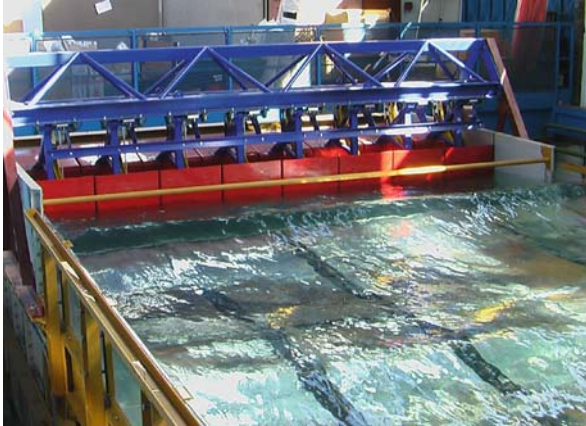
Fig. 5.18. Wave tank at the University of Manchester (small displacement piston paddle)
