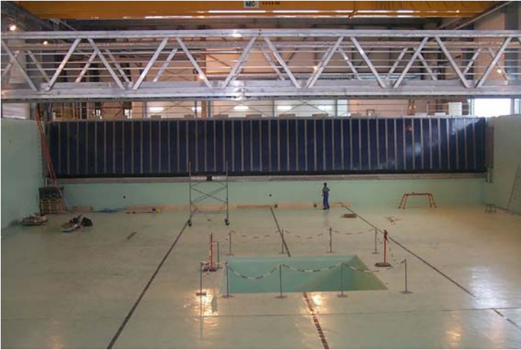
Fig. 5.20. 50 \times 30 \times 5 m wave basin at Ecole Centrale de Nantes
