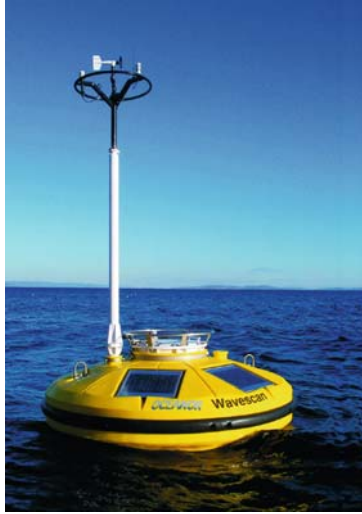
Fig. 4.11. The Wavescan heave/pitch/roll metocean data buoy has been used for directional wave measurements since 1984 and there are today more buoys than ever in operation, mainly in deep ocean, high current conditions. This buoy has, for example, collected data in the Agulhas current for one year, possibly the toughest environment in the world
