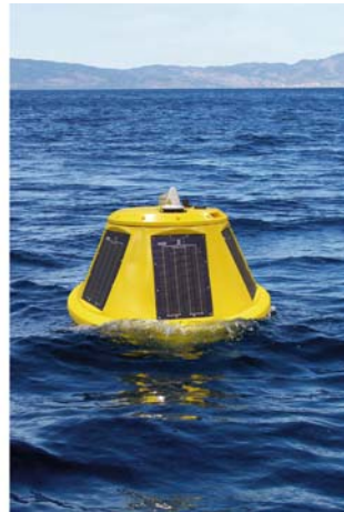
Fig. 4.12. The Seawatch buoy (left) and the Seawatch Mini mk. II (right) are used mainly for coastal monitoring. These buoys are examples of heave/displacement buoys. The mini buoy would normally be used for wave energy resource mapping where other metocean parameters such as wind data were not considered to be required
