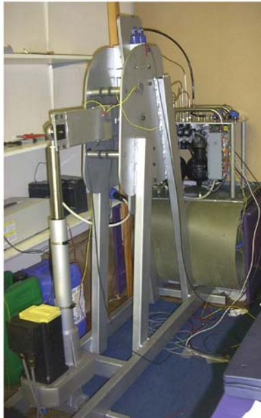
Fig. 5.29. Top: a fully assembled 7 th scale power pack positioned upside down from the orientation in which it is installed. The rams are connected to the manifold via flexible hoses fitted to ports extending through the hatch. Bottom: the 7 th scale test rig, fitted with a ballscrew actuator under position control, being used to test a 7 th scale power pack.
