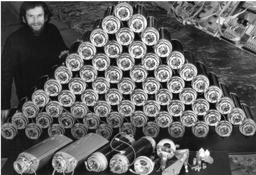
Fig. 2.10. David Jeffrey with the complete spine model. Beam elasticity could be varied electronically from the control bench. Two illicit generic absorbers can be seen, lower left
