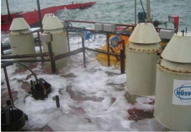
Fig. 7.80. Turbines in the reservoir of the prototype: The structure in the background is the siphon turbine, the grey towers are five of the six cylinder gate turbines, and the small devices in unpainted steel are two of the dummy turbines
