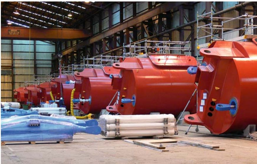
Fig. 7.63. Seven of the nine power conversion modules of the P1A machines lined up at the Fife Energy Park during initial assembly
