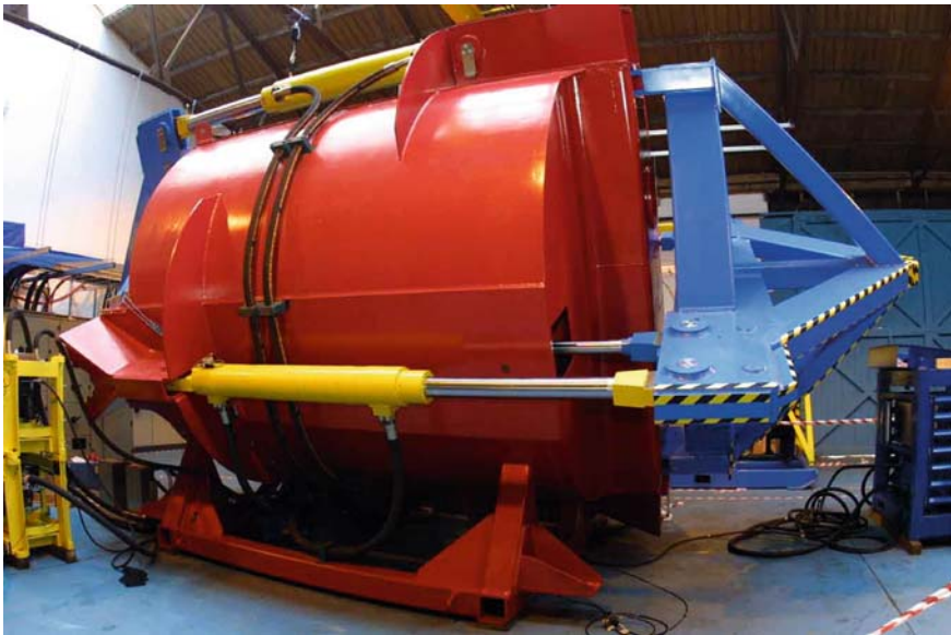
Fig. 5.30. The full-scale joint rig and associated control system: see the power take-off rams within the rig and the outer rams which are used for load simulation
