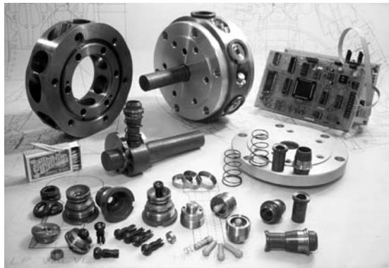
Fig. 6.57. The first Digital Displacement™ radial-piston pump built by Artemis Intelligent Power. Parts for the active low-pressure valve are in the left foreground. In the centre is a passive high-pressure check-valve. A 2 cc pumping module is at front right. The micro-controller is at back right. Photo: Artemis Intelligent Power Ltd
