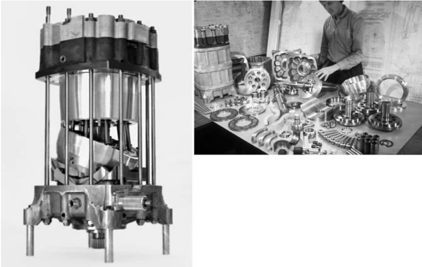
Fig. 6.50. Matthew Rea, in 1985, with parts that he and Carn Gibson made for a 600 kW Clerk high-speed motor. On the left, the motor is shown assembled without its case. The angled swash-plate is clearly visible (Photos: University of Edinburgh)
