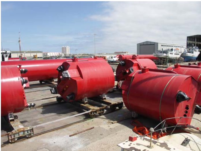
Fig. 7.65. Detail of the power conversion modules at the Peniche shipyard (Portugal)
