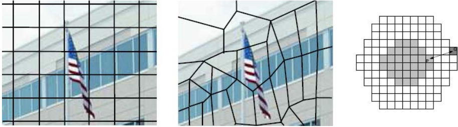
Fig. 3. Picture decomposition methods: regular grid (left), optimized Voronoi tiling (middle) and classification based on distance from arbitrary chosen points (right), [12]
