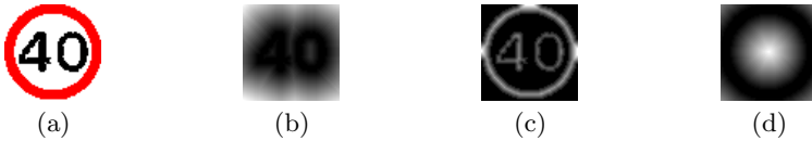
Fig. 3. Colour distance transform images: original discrete colour image (a), black CDT (b), white CDT (c), red CDT (d); darker regions denote shorter distance
