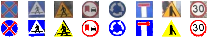
Fig. 2. Sample images obtained by sign detector before (above) and after (below) background masking and colour discretisation; 2 bits encode colours in each image
