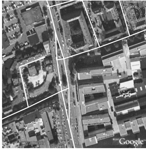
Fig. 2. A dual carriageway road intersecting with two normal roads. Geometries (white lines) of a commercial network dataset are shown against the background of an aerial view.
