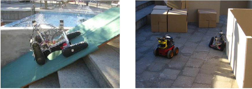
Fig. 2. Two different contexts that need different navigation strategies: on the left a “Lurkers” robot of Rescue Robots Freiburg facing a ramp, on the right together with an SPQR robot forming a group exploring an open space
