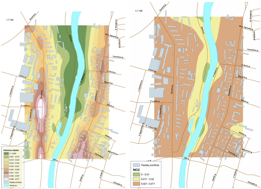
Fig. 2. Concentration levels of particle pollution ( left ) and zones of concentration of NO 2 ( right ) pollutions dangerous to people with respiratory disorders and asthma
