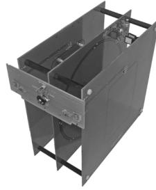
Fig. 2. Helmholtz assembly according to ISO/IEC 10373-6
