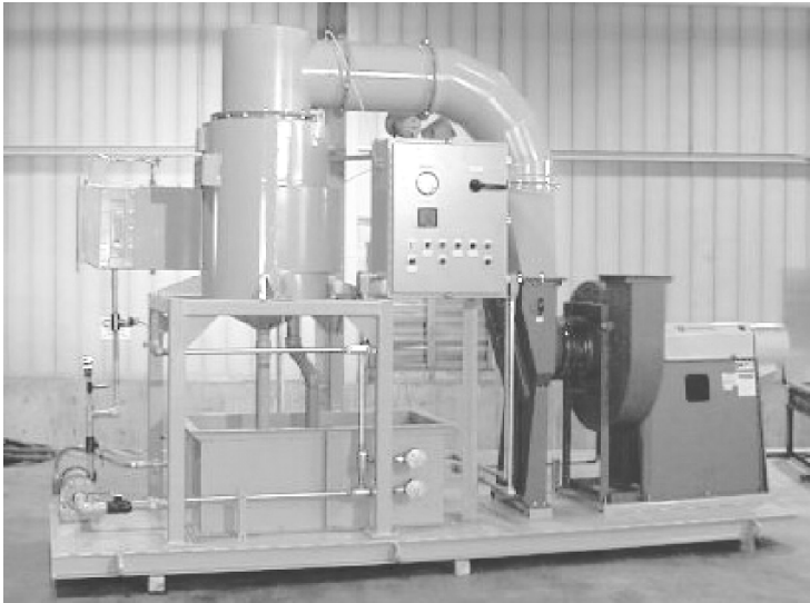
Fig. 13.3.6. A skid-mounted venturi scrubber/cyclone ensemble by Fisher-Klosterman, Inc.
