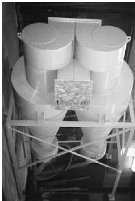
Fig. 15.1.19. A Beckert and Hiester twin cyclone dust collector featuring scroll inlets and gas outlets and helical roofs
