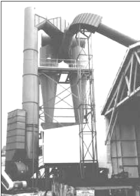
Fig. 12.1.10. A commercial installation consisting of a parallel arrangement of two cyclones sharing a common underflow hopper and overflow plenum (or 'header'). Note blower in bottom left-hand side of image 'pulls' gas through the cyclones. Also note the specially designed erosion-resistant elbow just ahead of the cyclones. Courtesy Fisher-Klosterman Inc.
