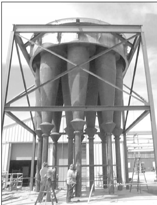
Fig. 16.2.8. A parallel set of 10 first-stage cyclones attached to the underside of the vessel head. Courtesy Fisher-Klosterman Inc.
