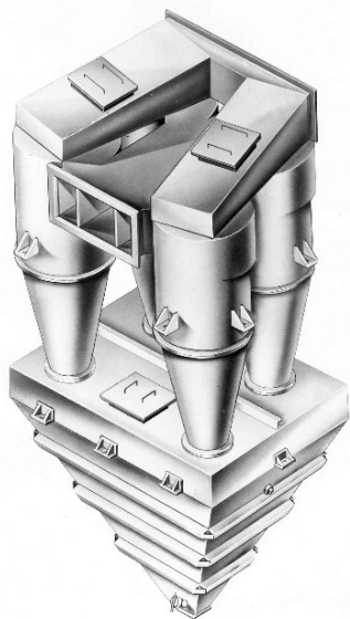
Fig. 16.2.5. A parallel arrangement of four cyclones sharing a common inlet duct and a common overhead and underflow plenum. Courtesy Ducon Technologies Inc.
