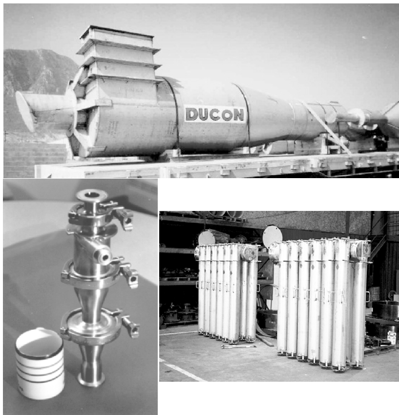
Fig. 1.3.2. A few examples of the variety of cyclone sizes and shapes used in commercial practice. Top photo courtesy of Ducon Technologies Inc., left photo courtesy of Fisher-Klostermann Inc., right photo courtesy of EGS Systems Inc.
