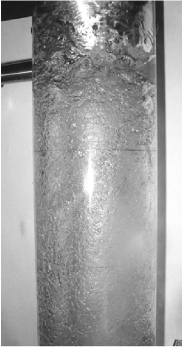
Fig. 4.2.3. A laboratory air/water cyclone showing wave-producing wall roughness. Photo by L. E. Stein
