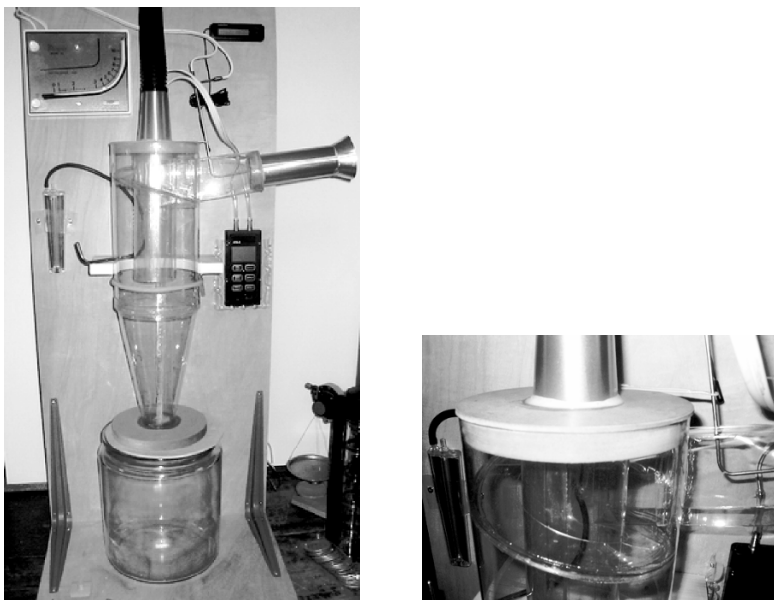
Fig. 15.1.21. Illustration of a helical-roof cyclone. Cyclone shown features one of the author’s (Stein) custom built versions of a Mini CV06 cyclone designed by Bill Pentz ( http://billpentz.com/woodworking/cyclone/index.cfm ) and built in clear PETG plastic (similar to Lexan ® but bendable) by Ed Morgano of Clear Vue Cyclones ( http://www.clearvuecyclones.com )
