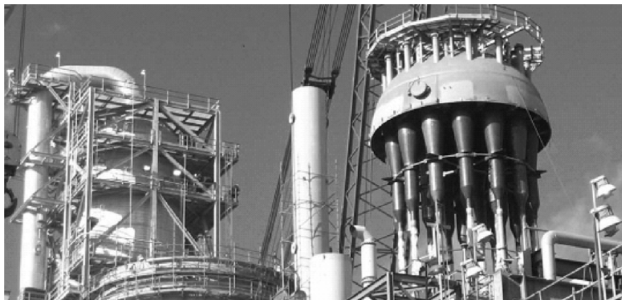
Fig. 1.3.5. A collection of two-stage cyclones suspended from the vessel head of a modern FCCU regenerator prior to installation. Photo courtesy of TapcoEnpro International
