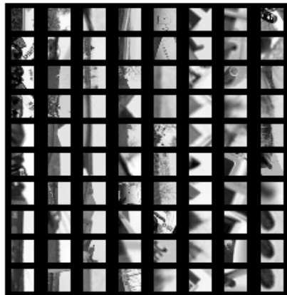
Fig. 5. Classification of feature vectors into 8 neighboring nodes of the growing neural gas. The columns represent the nodes. The entries of the columns are the last 10 feature vectors which were mapped onto them. The distance between the nodes is equivalent to the number of columns between them.
