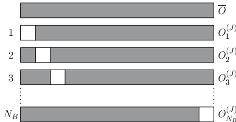
Fig. 4.7. Schematic sketch of the organization of Jackknife blocks. The grey part of the N data points is used for calculating the total and the Jackknife block averages. The white blocks enter into the more conventional binning analysis using non-overlapping blocks
