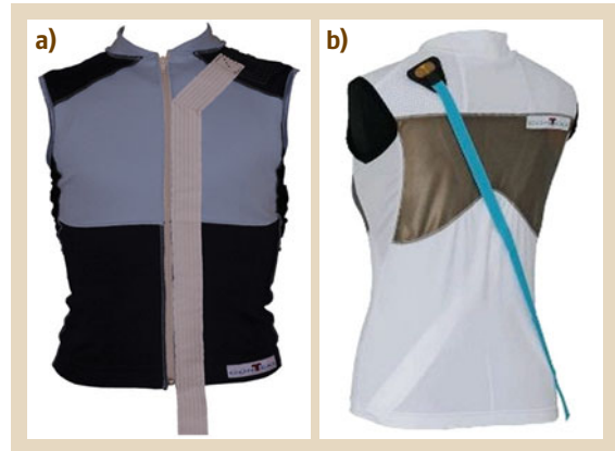
Fig. 73.15a,b ConText vest with textile-based contactless electrodes. (a) Prototype II, (b) final prototype (after [73.8])
