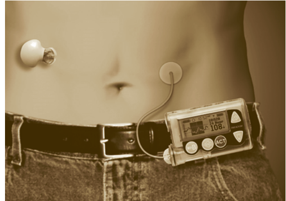
Fig. 67.18 The MiniMed Paradigm real-time system (after [67.50])
