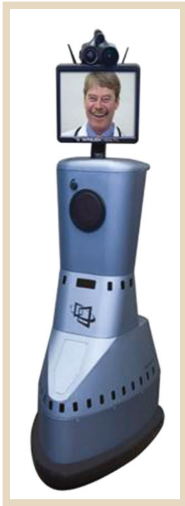
Fig. 70.15 RP-7 mobile robotic platform (InTouch Technologies, Santa Barbara, CA)
