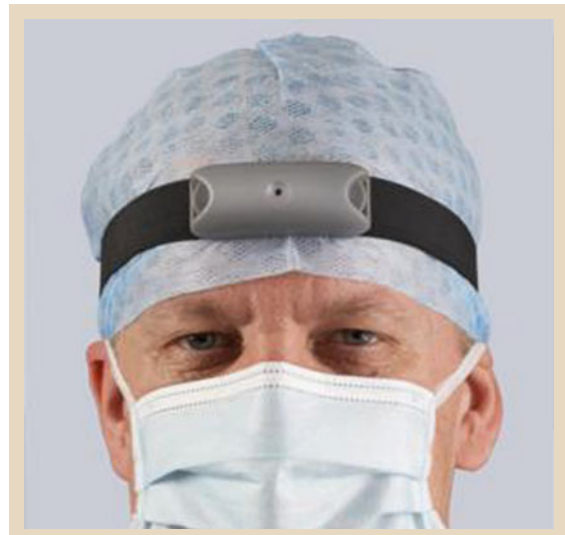
Fig. 70.8 Control unit of the FreeHand system, attached to the head of a surgeon by a rubber band (Prosurrgics Ltd., Bracknell)
