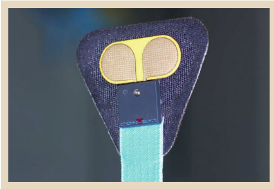
Fig. 73.18 Textile-based capacitive EMG electrode, Con-Text project (after [73.11])
