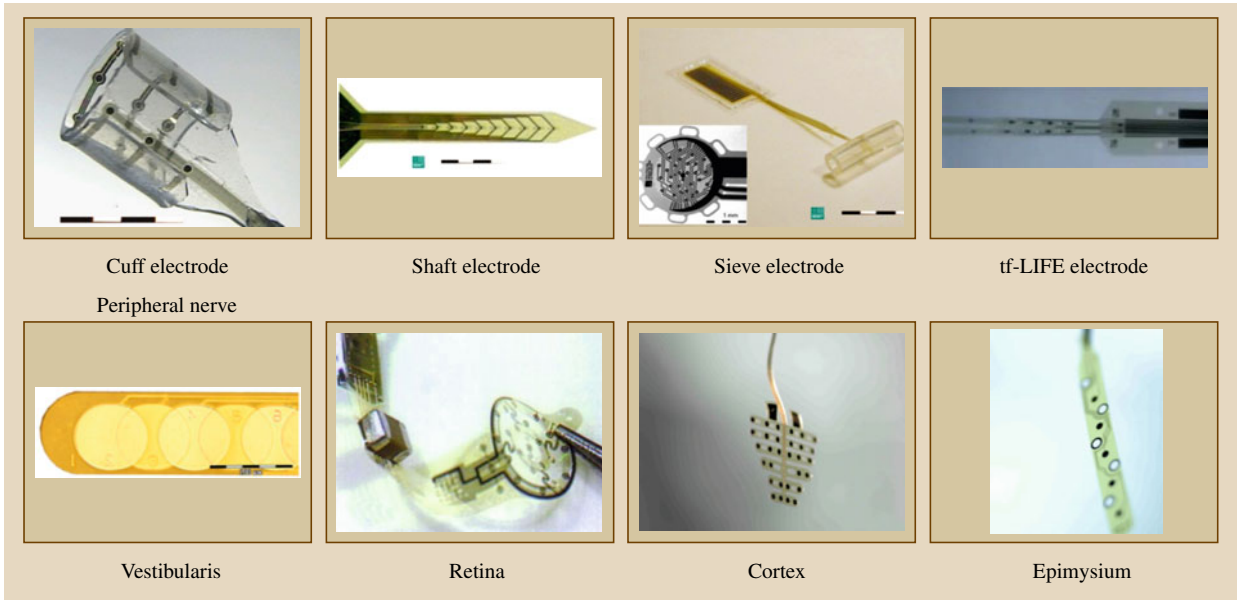
Fig. 39.4 Examples of flexible implantable microelectrodes made of polyimide
