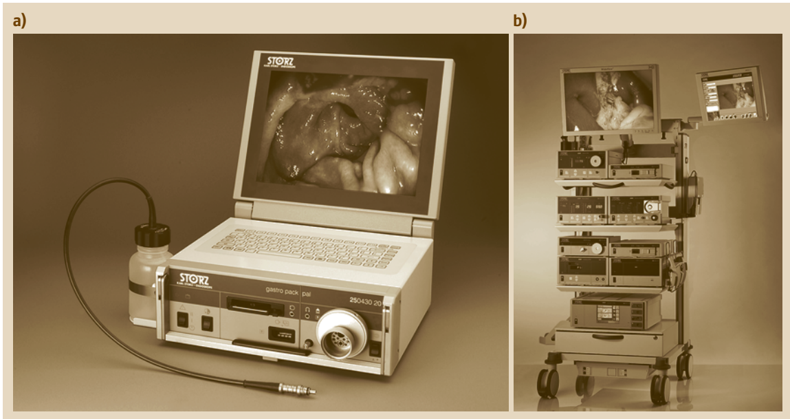
Fig. 19.9a,b Two different endoscopy workstations: (a) compact system for outpatient departments with camera control unit, light source, monitor, keyboard, and suction/irrigation pump (Gastropack), (b) equipment trolley for the operating theater additionally with HF surgery system, insufflator, and still image and video archiving system
