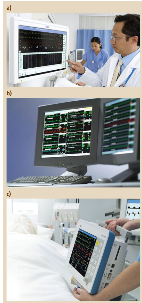
Fig. 47.1a–c Components in a modern monitoring system. (a) Widescreen information monitor ( foreground ) with integrated transport monitor (in the background on the docking station). (b) Central station for 16 patients. (c) Monitor is securely locked on a bed mount for transport (© Dräger Medical, Lübeck, Germany) ►
