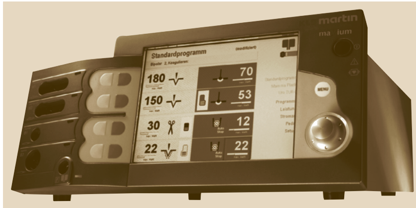
Fig. 34.2 Advanced HF surgical unit with a menu-guided user interface. The treatment parameters are clearly arranged on a screen next to the respective patient output
