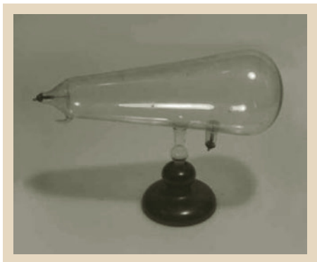
Fig. 35.3 Hittorf tube (cold cathode tube) (courtesy Electrosuisse Museum of Technology and Engineering, Fehraltdorf)
