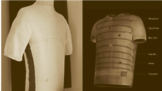
Fig. 74.14 SensatexSmart Shirt (Sensatex, Inc., Bethesda, MD)
