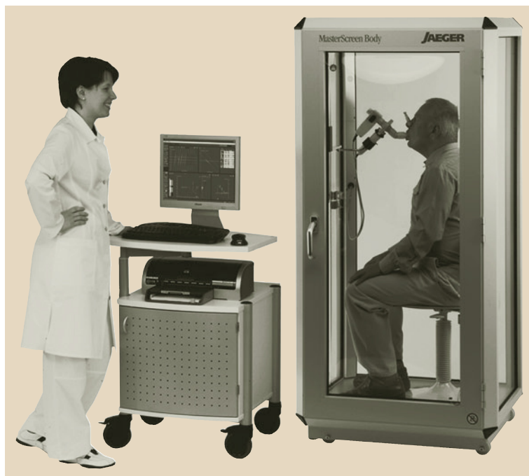
Fig. 8.8 Body plethysmograph (CareFusion 234, Höchberg, Germany)
