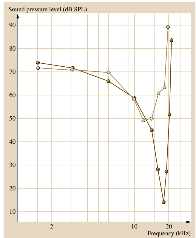
Fig. 12.4 Curves of constant basilar membrane velocity (0.04 mm/s) at one site of the basilar membrane, measured as a function of frequency with the Möbbauser effect of nuclear absorption of radiation. The comparison of results in a healthy ear ( full circles ) and an ear with damaged outer hair cells ( open circles ) of a guinea pig demonstrates the existence of a vulnerable frequency selective process that enhances the sensibility by about 40 dB within a restricted frequency range (after [12.6])
