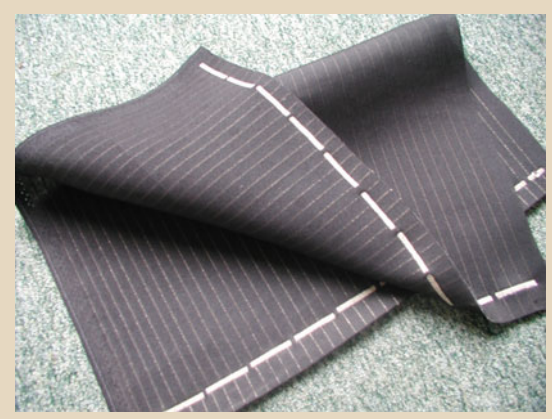
Fig. 73.27 Spacer fabric heating structure, heating threads integrated in the pole area (after [73.12], TITV Greiz)
