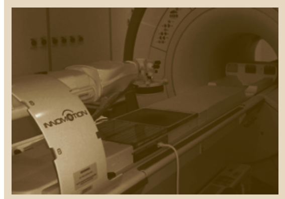
Fig. 25.21 Innomotion robot test setting on the ExAblate 2000 MRgFUS system (InSightec, Tirat Carmel, Israel), positioning the conformable bone system mobile FUS transducer ExAblate 2001 (IMSaT, Dundee, UK)
