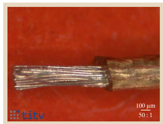
Fig. 73.10 Insulated ELITEX thread (TITV Greiz)
