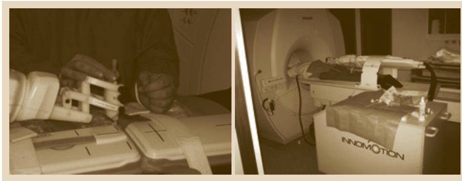
Fig. 25.10 Innomotion (Innomedic, Herxheim and KIT, Karlsruhe, Germany) MR-compatible robotic system (1.5 T GE HDX, Dundee (left), 1.5 T Philips Intera at Praxis Dr. Gert Lorenz, Gelsenkirchen, Germany)
