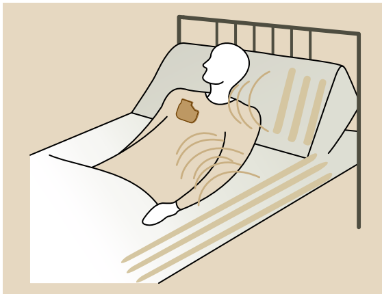
Fig. 74.12 Wireless power (power mattress and power pillow)
