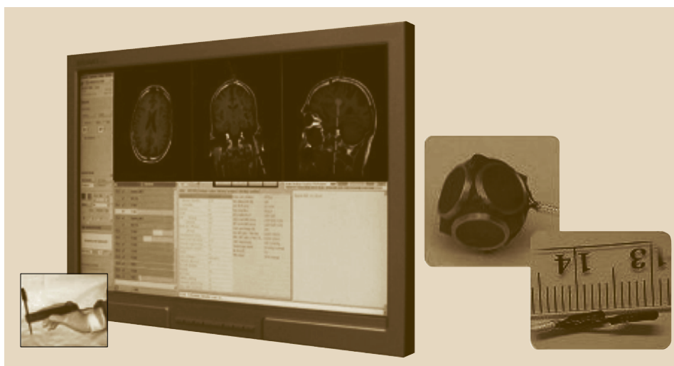
Fig. 25.7 Electromagnetic tracking in MRI enabled by a 3-D magnetic field sensor made from three orthogonal pick-up coils for a handheld guided tool and a microsensor with about 1.5 mm diameter for catheters (Robin Medical, Baltimore)
