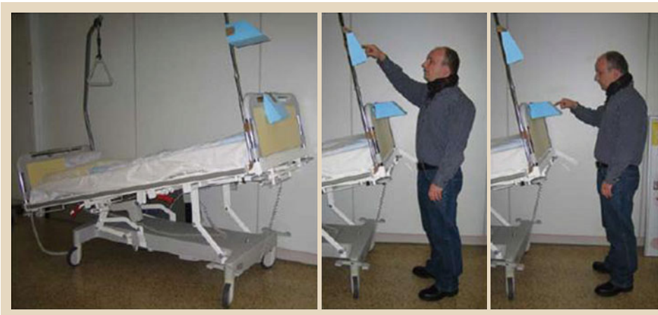
Fig. 6.11 With the aid of a rigid foam prototype, the ergonomically expedient installation on the patient bed is tested (after [6.20])
