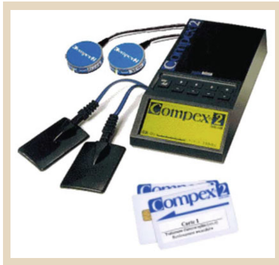
Fig. 44.2 Portable FES system with surface electrodes. This FES system is programmable using the memory chip cards and can make flexible stimulation patterns with four channels (after [44.38])
