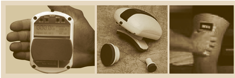
Fig. 14.4 Handheld dynamometer. Pictured is the Lafayette MMT System (Lafayette Instrument Company, Lafayette)
