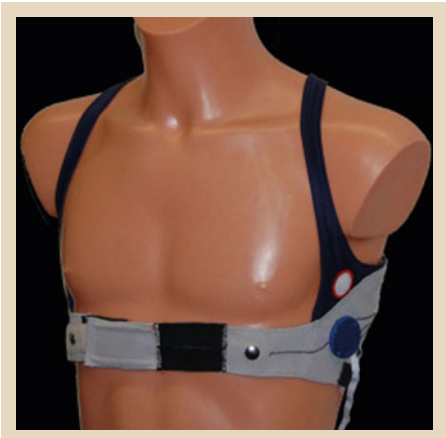
Fig. 73.14 MμGuard monitoring vest monitoring vest with silicone based dry contact electrode (after [73.10])
