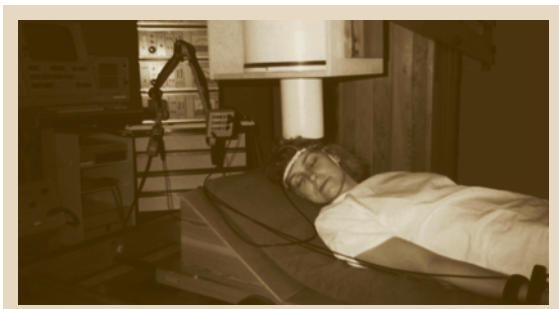
Fig. 46.20 Simultaneous registration of a somatosensorily evoked potential and the somatosensorily evoked magnetic field after stimulation of the median nerve of the right hand
