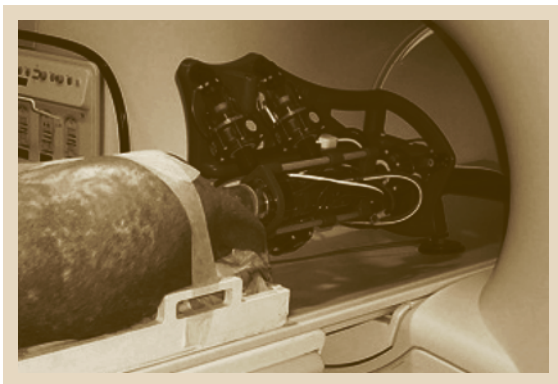
Fig. 25.15 Johns Hopkins MR-compatible robot in an animal procedure for prostate interventions (after [25.32])
