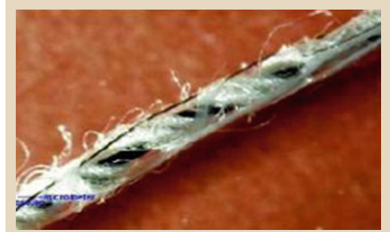
Fig. 73.13 Core mantel thread construction of textile and metallic components (TITV Greiz)
