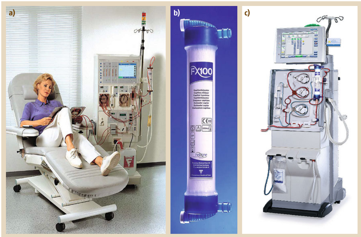
Fig. 31.1a–c Blood purification by hemodialysis is achieved in patients with kidney disease when blood is passed and filtered extracorporeally through a dialyzer. Treatment parameters, such as blood flow, dialysate flow, blood pressure, blood volume, pH, and the performance parameters, can be assessed and appropriately monitored by the dialysis machine. Patients (a) undergo this procedure three times per week for 4 or more hours nearly as a rule. Dialyzers (b) are the key functional elements of blood purification systems. Dialysis machines (c) (5008 machine from Fresenius Medical Care) are able to control a patient-specific therapy with the assistance of feedback systems. Even highly efficient blood purification systems, such as hemodiafiltration, can be operated cost-effectively, as the machine offers online availability of the necessary substitution solution directly from the dialysis fluid as a standard
