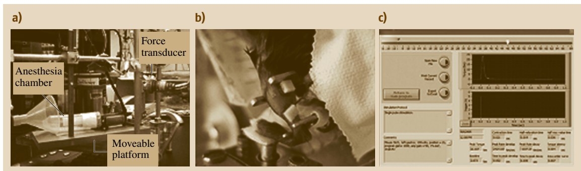
Fig. 14.16 (a) Device setup employed for noninvasively studying leg force properties in a mouse, (b) leg setup and electrode placements, and (c) online LabVIEW program display of measured forces (after [14.50])
