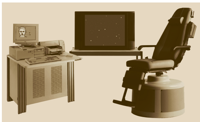
Fig. 11.9 Measurement station for the examination of the nystagmus after optokinetic stimulation with moving patterns on a television and vestibular stimulation using different movement patterns of a swivel chair (courtesy Jaeger Tönnies GmbH, Würzburg)
