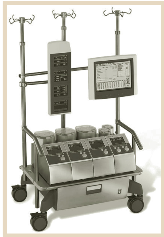
Fig. 32.6 Industrial heart–lung machine with panel PC and data management system (Sorin Group, Munich)
