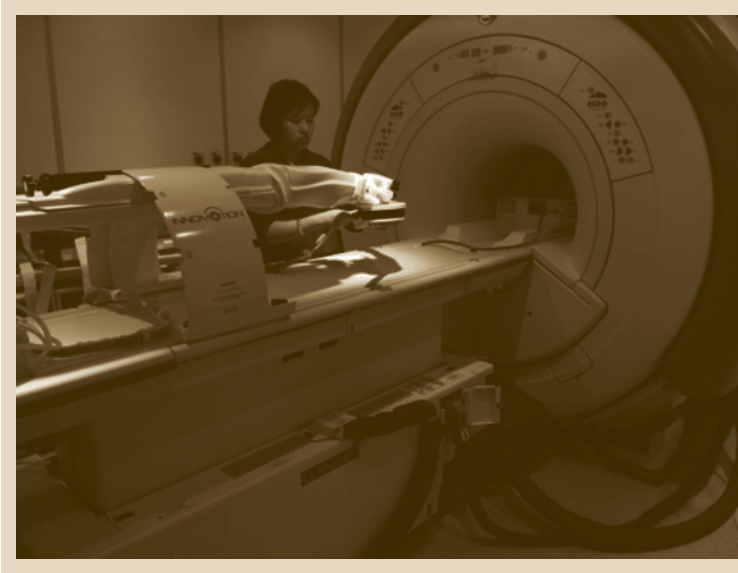
Fig. 25.16 MR-compatible robotic system in combination with a MR-guided focused ultrasound system (ExAblate 2001, InSightec, Tirat Carmel, Israel)
