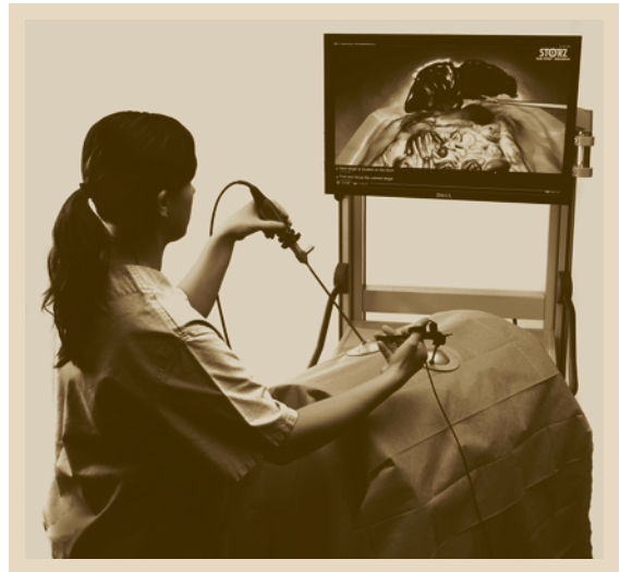
Fig. 19.19 Virtual MIS simulator for laparoscopic interventions
