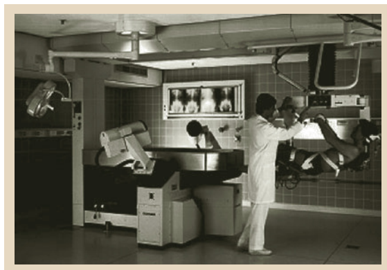
Fig. 33.1 The first series lithotripter Dornier HM3 was introduced in 1983. The patients were treated by the spark-gap source in a large bathtub filled with degassed water. Targeting was done using two crossed x-ray tubes
