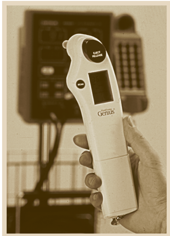
Fig. 50.4 Digital thermometer for measurement in the external auditory canal (courtesy of Johnson & Johnson, USA)
