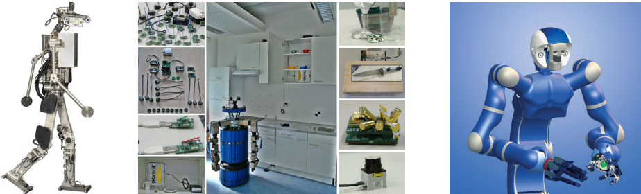
Fig. 2. Demonstrator platforms humanoid robots. The COTESYS cluster investigates ways to equip the walking machine Johnnie (left, ©Prof. Ulbrich, TUM) and its currently developed successor Lola and Justin (right, ©Prof. Hirzinger, DLR), a humanoid upper body system for two handed manipulation, with cognitive capabilities. Intermediate research platforms are existing mobile robots with manipulators such as the B21 robot depicted in the middle acting as a kitchen assistant. Scenarios in which cognitive capabilities will be demonstrated include household work, party service, and shopping.
