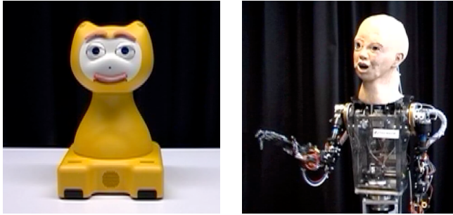
(a) iCat, a desktop robot developed by Philips Research. (b) BARTHOC, an anthropomorphic robot.
