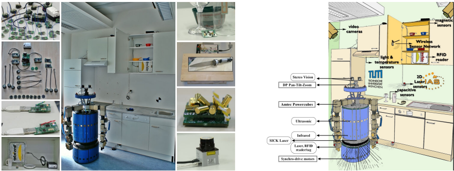
Fig. 6. The Assistive Kitchen containing a robot and a variety of sensors. The sensors provided by the environment (left) in the form of a sensor network include laser range finders, RFID tag readers, force and acceleration sensors, and CCD cameras. The mobile manipulation platform is equipped with two robot arms with grippers, and various sensors, most notably a stereo camera unit and small laser range sensors mounted on the robot grippers.
