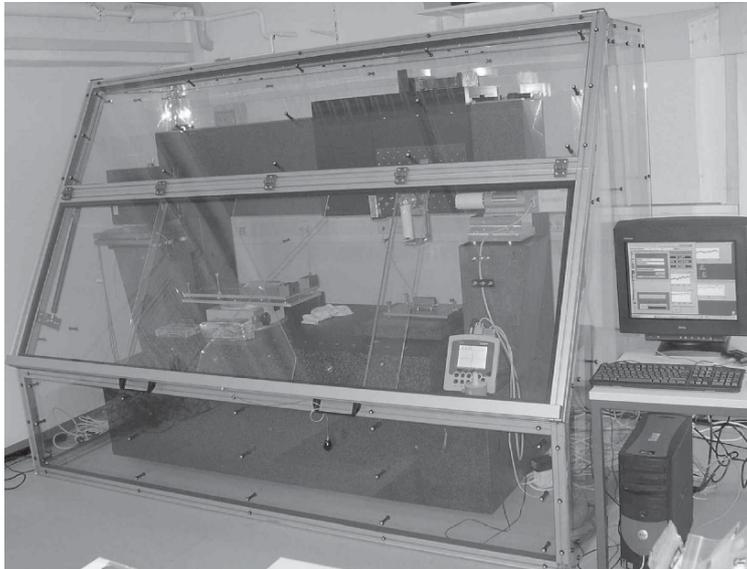
**Fig. 11.1.** The nano optic measuring machine NOM at BESSY. To insure stable environmental conditions the instrument is enclosed in a double walled housing
