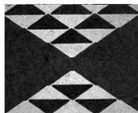
**Fig. 21.6.** Optical micrograph of the present clessidra lens. The contrast was adjusted such that the resist surface is particularly revealed
