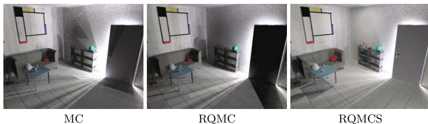
Fig. 5. Visual comparison for the test scene “Invisible Date” using 300 chains for simulation. The only lightsource is not visible as it is placed on the ceiling of the neighboring room. Due to the better distribution of the photons randomized quasi-Monte Carlo (RQMC) outperforms Monte Carlo (MC) visually, as can be seen by the reduced shadow artifacts. RQMC with sorting (RQMCS, using 256^3 voxels for the bucket sort) is even superior as more photons made it into the second room and even the back of the door is lit very well.
