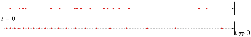
Fig. 1. Samples along a ray x_0 + t\omega for t \in [0, t_{\partial V}] : transformed random points (top) and transformed equidistant points (bottom). The latter yield a better distribution for the initial points in Algorithm 1.
