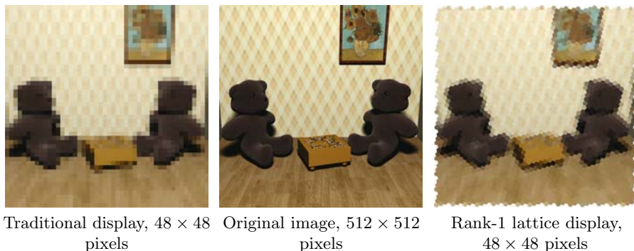
Fig. 13. Comparison of rank-2 (left) and maximized minimum distance rank-1 lattice (right) displays at identical pixel resolution for approximating the high resolution image in the middle.
