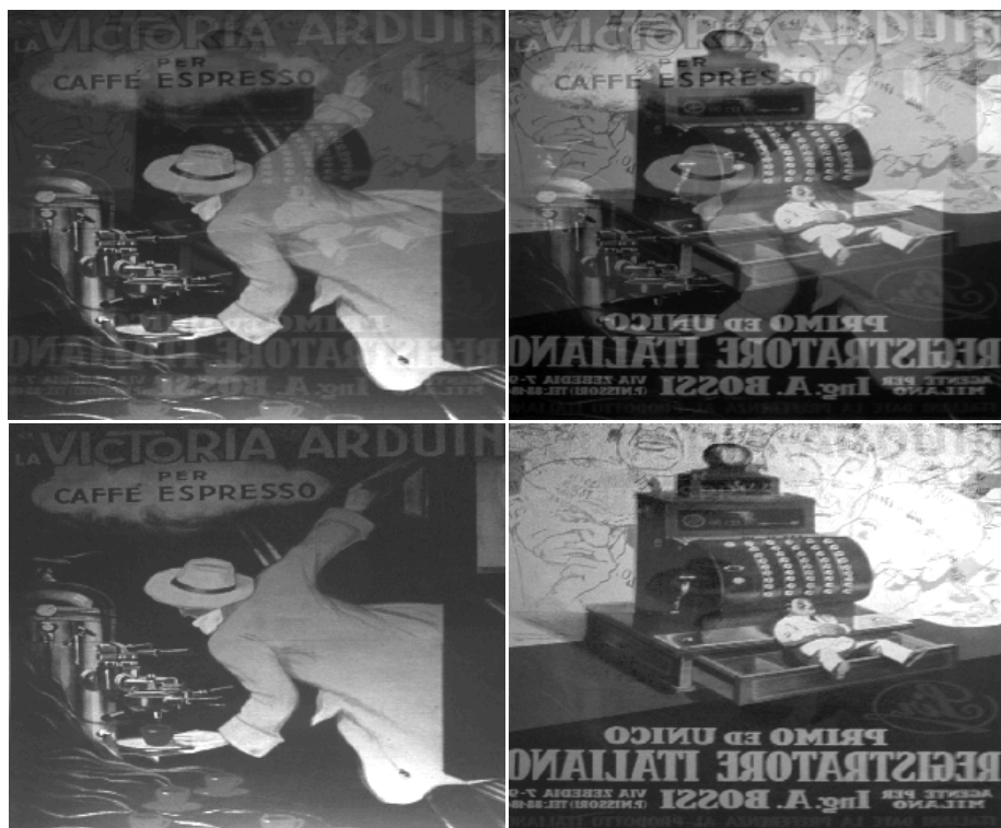
Fig. 3. Results of separating the real mixtures: [Top] The mixtures. [Bottom] Estimated separated sources.
