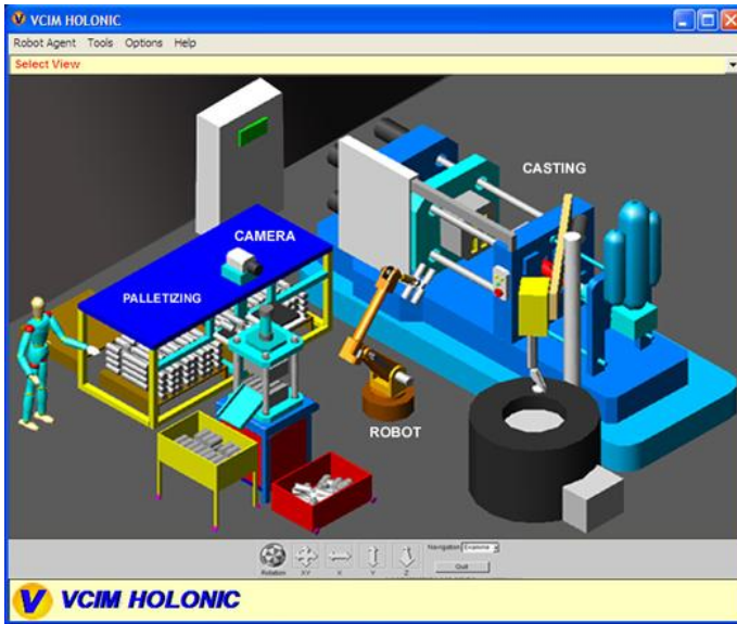
Fig. 3. A snapshot of the developed prototype tool VCIM-HOLONIC, employed for the implementation into holonic control of a fully automated die-casting cell
