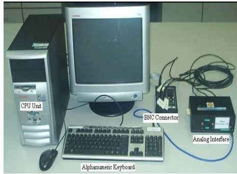
Fig. 1. Integration of biometric authentication system component
