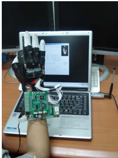
Fig. 4. The proposed glove and KFS recognition system
