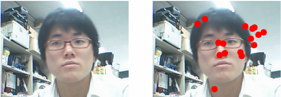
Fig. 3. Face tracking using pyramidal Lucas-Kanade feature tracker
