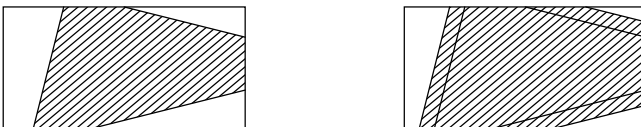
Fig. 1. Comparison of (MPC) with the relaxed version (MPC_{c,\epsilon}) where B \subseteq \mathbb{R}^2 is a rectangle with 3 linear constraints; hatched areas indicate the feasible regions
