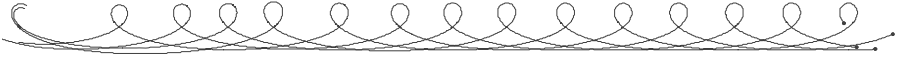
Fig. 7. Trajectories of 4 UAVs orbiting a moving target trace out routes similar to those in this figure
