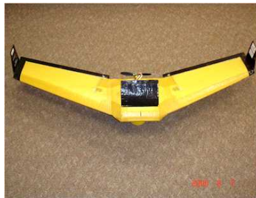
Fig. 14. Procerus UAV with 60” wingspan used for live flight experiments
