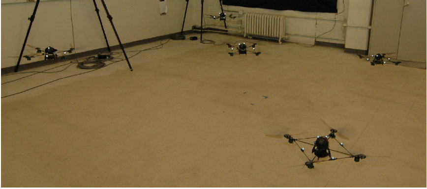
Fig. 1. Five vehicle coordinated flight test on MIT's RAVEN [8]
