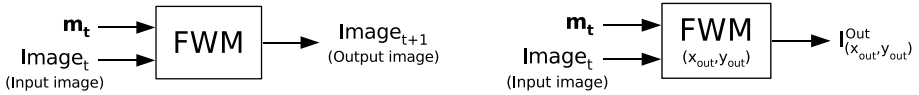
Fig. 1. Left: Visual forward model (FWM). Right: Single component of a visual forward model predicting the intensity of a single pixel (x_{\text{out}}, y_{\text{out}}) of the output image.
