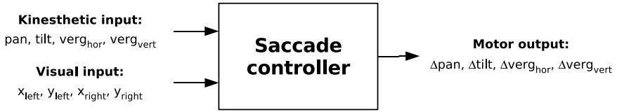
Fig. 7. Input and output of the saccade controller (for details see text)
