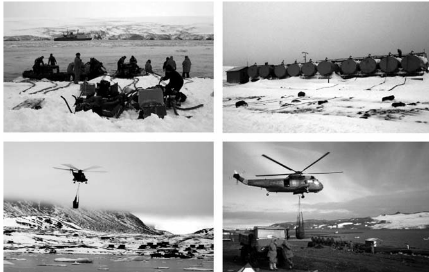
Fig. 12.1 Refueling activities in Antarctic Stations require transport of fuels from logistic ships to storage tanks by boat, helicopter, and/or pipeline. These operations are essential but imply an important environmental risk
