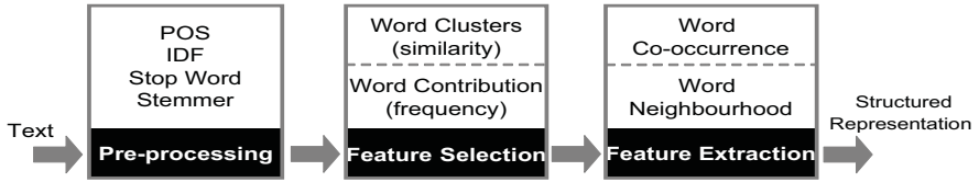
Fig. 1. Processing unstructured text to create structured representation
