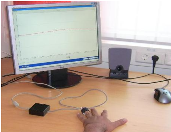
Fig. 1. Taking finger temperature measurement using a temperature sensor
