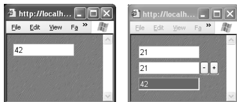
Fig. 1. (a) A single integer editor. (b) Display the sum of two integer input fields.
