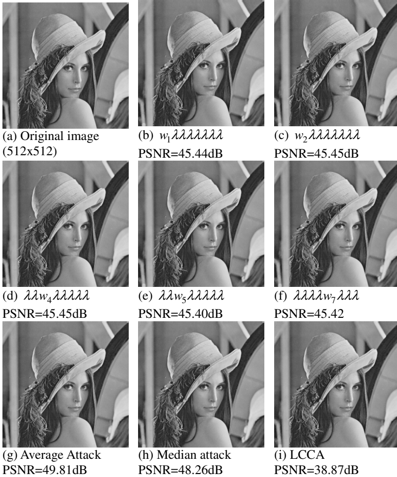
Fig. 4. (a) original image, (b-f) five fingerprinted images, collusion after (g) average attack (h) median attack, and (i) LCCA. (Repetition factor = 2, number of marks = 8).
