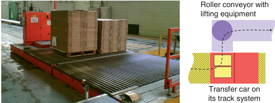
Fig. 1. Left: Two stacks on a deck position of an automated guided transfer car at an intersection to a roller conveyor [33]. Right: Schematic representation of the element in the left figure. The change of the movement direction on the conveyor is performed by a short roller conveyor with lifting equipment (so-called chain crossover) and is marked by a circle.
