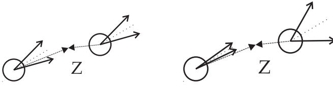
Fig. 9. Effect of different values of the internal parameter \mu_i on the turning behavior in the Centripetal Ant Model; Z is the center of the nest; (left) for large \mu_i there is only a slight difference between moving from or to the center; (right) for small \mu_i the turning angle becomes significantly smaller the larger the angle between actual moving direction and the vector to the center
