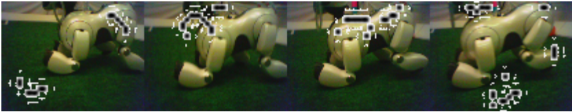
Fig. 7. Four sequential frames from a test run. The robot in the images is moving to the left at full speed. Overlaid black squares on the image indicate the discontinuities found by the postprocessing algorithm; when enough of these squares appear in a sector of the image, the system concludes that this sector contains motion.
