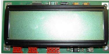
Fig. 8. “LC-display board”: expansion board with LC-display
