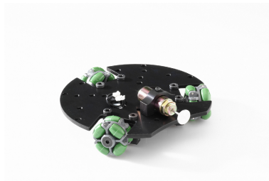
Fig. 13. Omnidrive platform with three omnidirectional wheels
