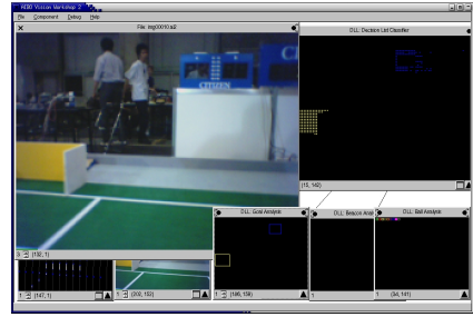
(b) The blue timer appears as a goal with the yellow goal
