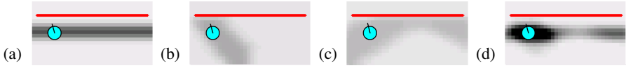
Fig. 4. Likelihood of positions given the observed line using (a) the Hough parameters only, (b) the \bar{u} value, (c) the \sigma(u) value and (d) all four parameters (the darker the more likely)
