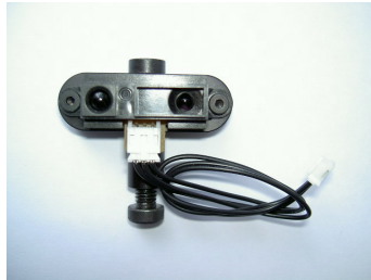
Fig. 5. Exemplary sensor bearing for an IR distance sensor
