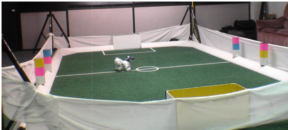
Fig. 4. The training environment during the gait parameter optimization experiment. The Aibo records how long it takes to move between two beacons. It also records the average accelerometer values, the average difference in the position of the centroid of the beacon and the center of the image, and the average slope of the beacon in the image.
