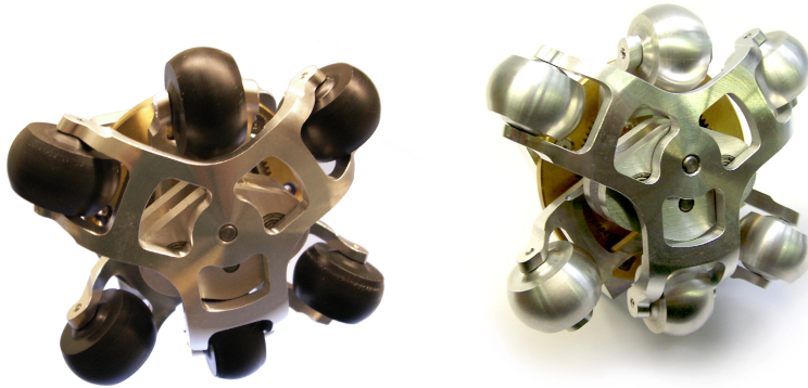
Fig. 8. Our first two Reuleaux omnidirectional wheel prototypes
