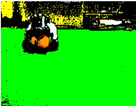
Fig. 7. The left figure shows how our vision system recognizes a ball when the other robot holds it. The ball looks to be smaller than it is, because a part of it is hidden by the partner and its shadow, resulting in an estimated distance to the ball that is further away than it really is. The right figure plots the estimated values of the both the distance x and the velocity dx , when the robot kicked the ball to its partner, the partner trapped it, and then the partner kicked it back. When the training partner was holding the ball under its head though (the center of the graph), we can see the robot obviously miscalculated ball's true distance.
