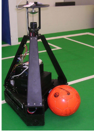
Fig. 1. The omnidirectional robot equipped with a digital color camera and a hyperbolic mirror on the top
