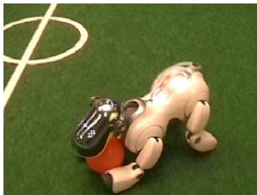
Fig. 1. An Aibo with control of a ball. Achieving this position without knocking the ball away in the process is a challenge; our learning method allows the Aibo to do this more reliably without sacrificing walking speed.
