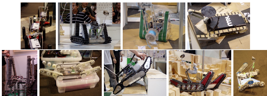
Fig. 1. Flippers as additional tracks that can change their posture relative to the main locomotion tracks are a very common approach to allow for a flexible footprint. The general advantages of this locomotion principle is for example indicated by the many teams that chose this approach for their robots. Some examples from RoboCup 2005 are shown above.
