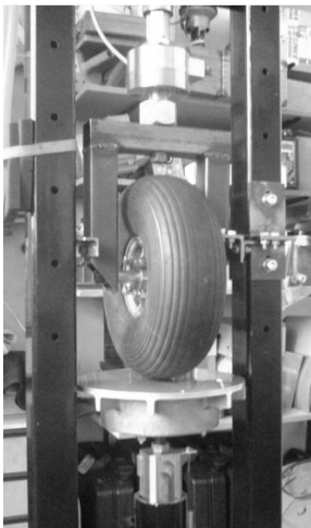
Fig. 2: Tested tyre in tester
