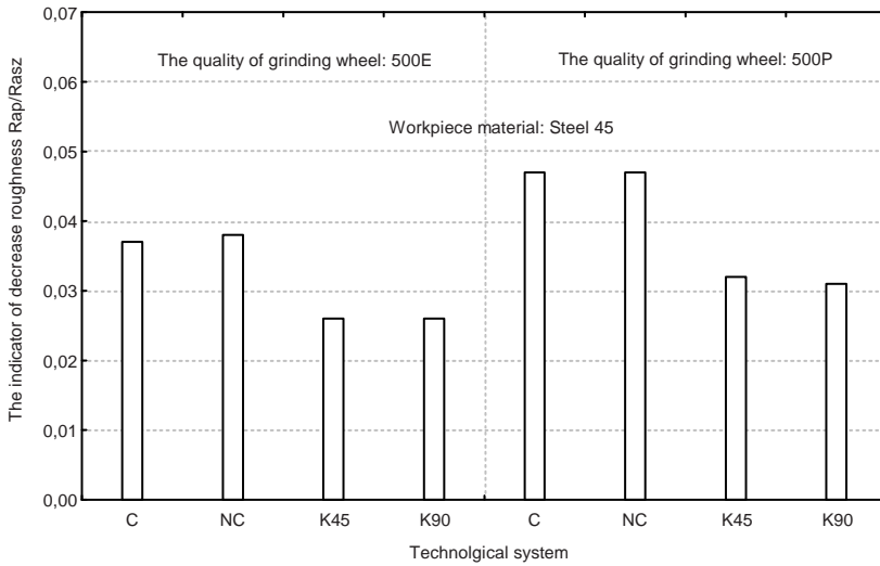
Fig. 3. The influence of technological system on the indicator of decrease roughness Ra_p/Ra_{sz} of the steel 45 surface which was polishing the grinding wheels 500E and 500P of polyurethane bond
