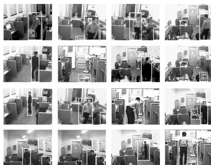
Fig. 4. The results of multi-target detecting and classifying, where the solid rectangle represents human target and the dashed rectangle represents non-human target
