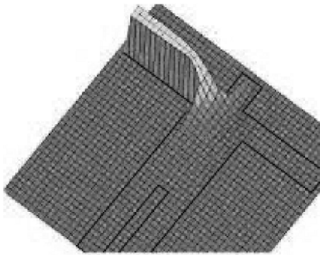
Fig. 3 Surface plot of impedance sensitivity for the right arm region
