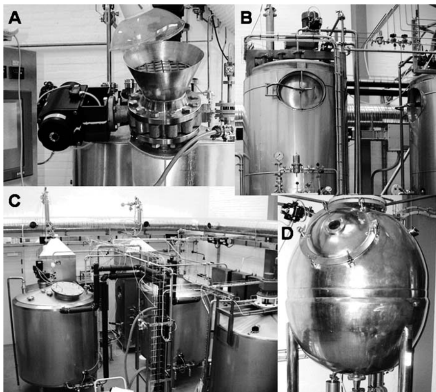
Fig. 5 The pilot plant at DTU. a Inlet. b Fermentation tanks (2700 L each). c Fermenters and holding tanks. d Distillation tank
